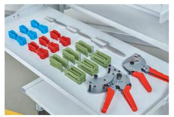
Toolkit with various-sized crimp clamps, crimping tongs, cutting tool and opening tools
