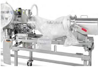
The dosing screw can be replaced inside the film liner under containment conditions. To do so, the appropriate tools are first passed into the liner beforehand.
