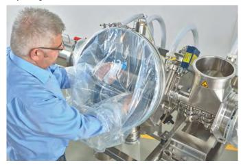
The inspection hatch can be opened using the gloves attached in the film liner and the screen basket can be inspected by turning it.
