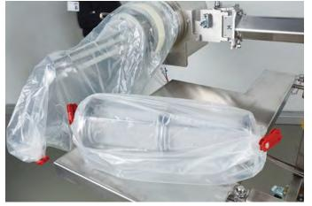
The contaminated screen basket is replaced under containment conditions with a cleaned screen basket using a film liner and the crimp fasteners. The machine operator and the environment remain protected from contamination during the entire procedure.
