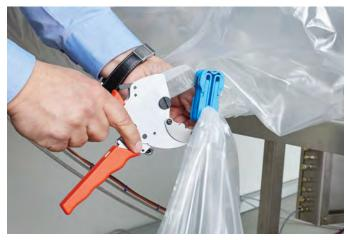
To seal the film liner at a specific place, the crimp clamp is pulled over the bag by hand and compressed using special crimping tongs. After this the crimp can separated using a cutting tool.
