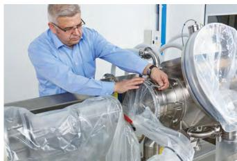
After the screen basket has been replaced, the contaminated sections of film are drawn inside the new liner into the side pockets. After crimping off the pockets, they can be disposed of together with their contents.
