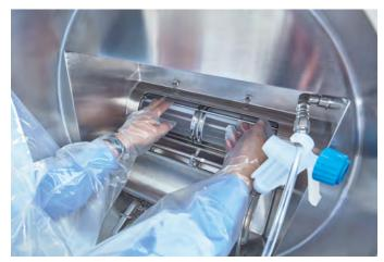
After the hatch is closed again, a cleaning gun can be used to bind the dust that clings to the hatch. The cloth used for wiping is disposed of in a side pocket.
