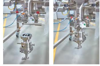
For wet cleaning, the coarse material container is replaced with a cleaning model in just a few steps. This is fitted with a cleaning head and a connection for a drainage line.
