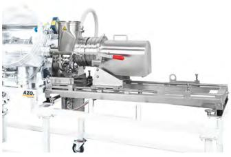
The entire dosing module, consisting of drive, dosing screw, product inlet and extractor slide, can be replaced in order to attain different performance figures. To do so, it is separated from the rest of the screener using a changeover rail.
