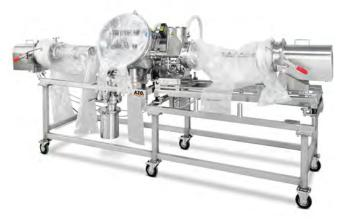
The screener is fitted with film liners. This make it possible to replace both the contaminated screen basket with a cleaned one and also the screw feeder in the dosing module under containment conditions.
