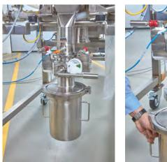
The coarse material container is connected to the machine via splitvalve technology. The coarse material accumulated in the hopper can then be disposed of under containment conditions or fed back into the production process.
